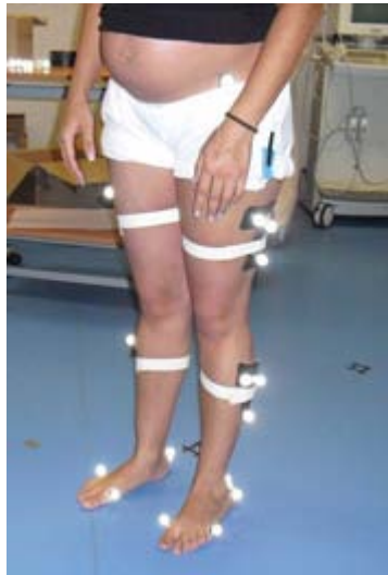
Figure: Reflective markers placed on anatomical landmarks
